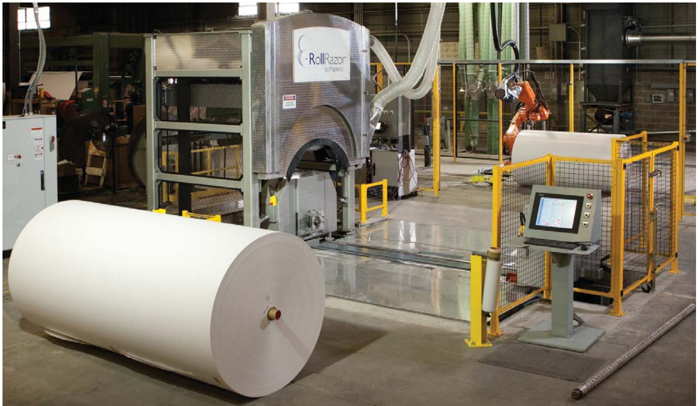
The Norkol system combines RollRazor cutting technology with an ABB Robot and ATI Force/Torque Transducer
